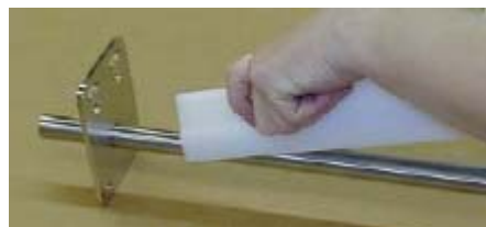
Exhibit 7: Blade Installation Method
